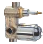
F4030101 Concealed body for high flow single lever, concealed diverter system consisting of 45 mm cartridge with button Assembly, Cartridge Sleeve (but without operating lever, wall flange and tip ton knob)
