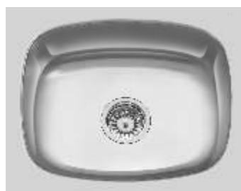
DORA Single bowl sink manufactured from 1.0 mm thick 304 grade stainless steel Size: 510 x 430 mm (20" x 17") Depth: 203 mm (8") Installation: Top mount
