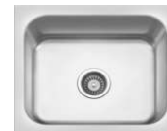
LILAC Single bowl sink manufactured from 1.0 mm thick 304 grade stainless steel Size: 510 x 430 mm (20" x 17") Depth: 205 mm (8") Installation: Top mount
