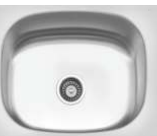
QUEEN Single bowl sink manufactured from 1.0 mm thick 304 grade stainless steel Size: 610 x 460 mm (24" x 18") Installation: Top mount
