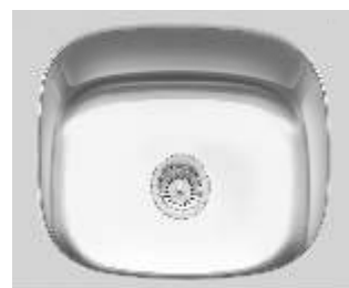
DALLAS LITE Single bowl sink manufactured from 0.8 mm thick 202 grade stainless steel Size: 610 x 455 mm (24" x 18") Depth: 255 mm (10") Installation: Top mount Cat. No. B4621101 - Gloss finish Cat. No. B4621101 - Matt finish
